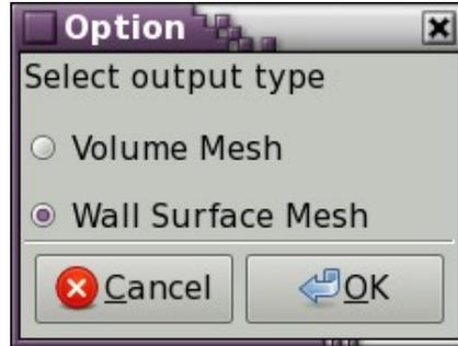
By clicking the sub-menu 'Postprocess Data', an option window pops up. In this window, there are two options with the help of which user can write the volume data or wall surface data.
