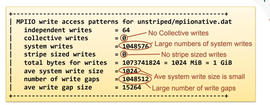
This is a simple example for 3D decomposed array. Independent MPI-IO writes are used in place of collectives.
