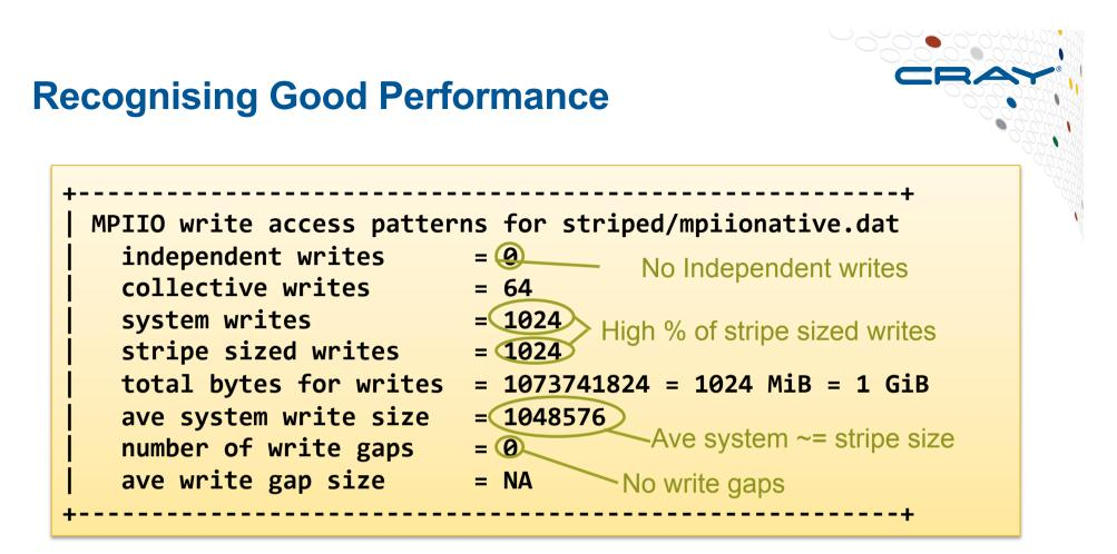
This same simple example for 3D decomposed array. Now using collective MPI-IO writes:
