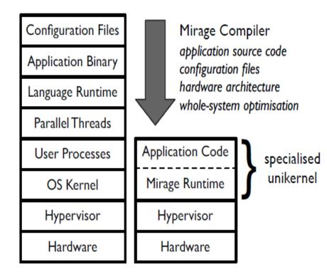
Unikernel system abstraction layers as compared to application services deployed over general purpose OS residing in a VM.
